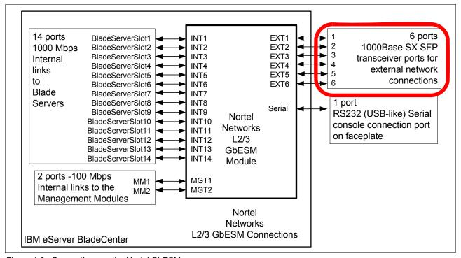
Figure 4-6 Connections on the Nortel GbESM
